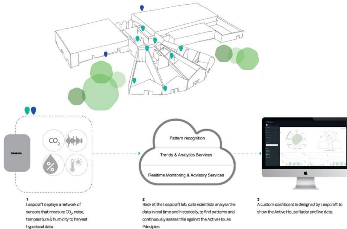
From Green Solution House to Leapcraft's Lab—harvesting data, robust and reliable cloud infrastructure, data analysis and custom builds for visualisations deliver a human-readable sensemaking of sensors.
